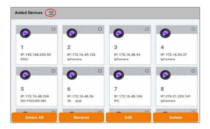
Tap to display the buttons as shown above. Select the device and then tap "Edit" to modify the username and password of the added device; tap "Delete" to delete the device.
