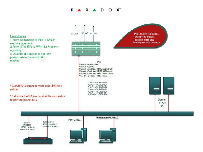
Figure 1. Network isolation using VLAN.
