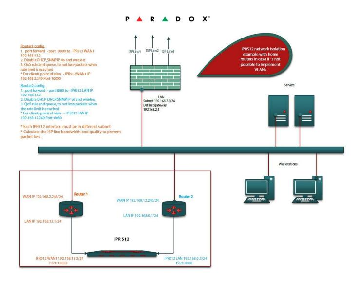
Figure 2. Network isolation using routers.
