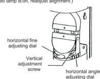
NOTE: After completion of optical adjustment, ensure that both filters on the receiver are replaced to their original position behind the mirrors.
