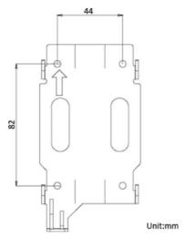
Figure 3-1 Wall Mounting Plate
