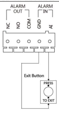
Figure 2-4 Exit Button Wiring
