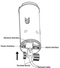
**Figure 3-3 Insert Terminals and Network Cable**
