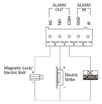
Figure 2-2 Door Lock Wiring
