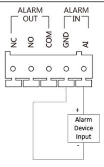
Figure 2-5 Alarm Device Input Wiring
