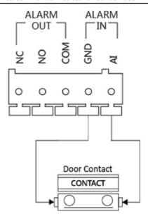
Figure 2-3 Door Contact Wiring
