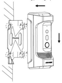
Figure 3-5 Hook the Doorbell to the Plate
