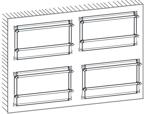
Figure 2-5 Mount Brackets on the Wall
