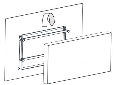
Figure 2-8 Mount Display to Bracket
