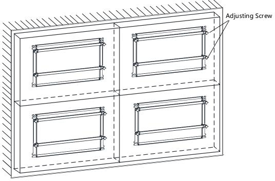
Figure 2-10 Adjust Displays
