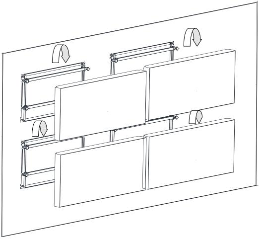
Figure 2-9 Mount Displays to Brackets
