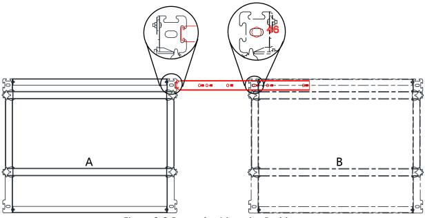
Figure 2-3 Determine Mounting Position
