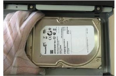
3. Put the HDD into the Device.
