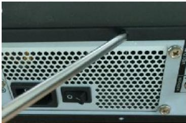
1. Loosen the screws on the panel and remove the cover.
