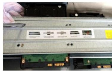
2. Fix the HDD(s) onto the bracket. Remove the top bracket if you want to install HDD to the bottom bracket.
