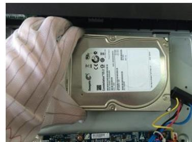
3. Place the HDD onto the Device.
