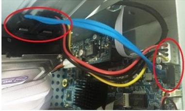
7. Use the HDD cable and power cable to connect HDD and mainboard.
