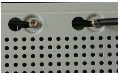
4. Turn the device to see the back side of it. Aim the screws of the HDD at the holes on the back of the
