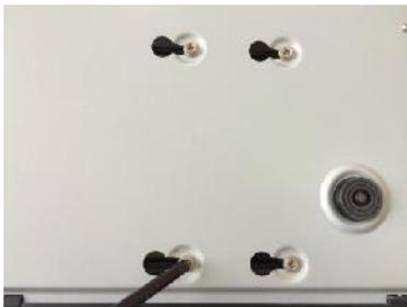
4. Turn the device to see the back side of it. Aim the screws of the HDD at the holes on the back of the device, and then fix the screws.
