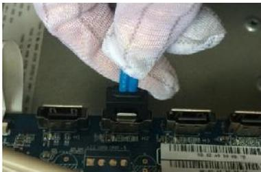
4. Connect the other end of HDD cable to the mainboard
