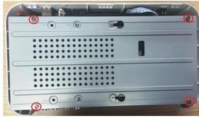
8. Install the bracket back and then fasten the screws.
