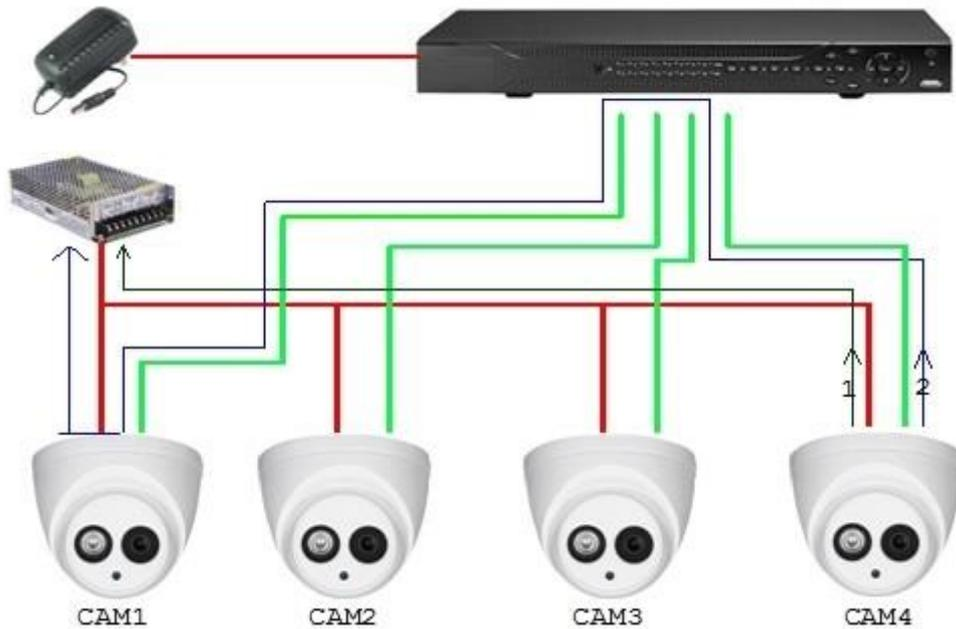
There are two paths for the power output of CAM4, return path 1 and return path 2. Reflow 2 first flows to CAM1, and then flows to the power supply from power supply ground of CAM1. In this way, the reflow of power supply ground CAM4 affects the video ground of CAM1, resulting in interference stripes on the screen. And CAM4 also interferes with CAM2 and CAM3.
