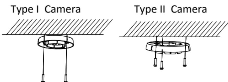
Figure 2-3 Attach the Mounting Base to the Ceiling
