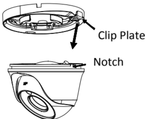
Figure 2-6 Disassemble the Camera
