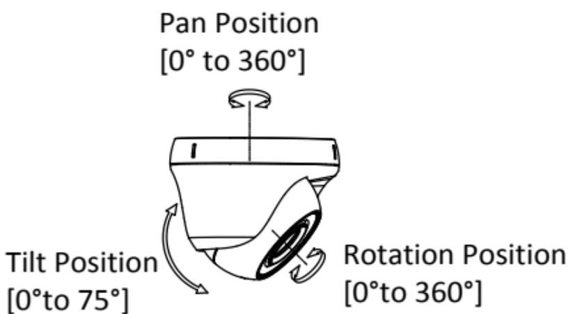
Figure 2-5 3-axis Adjustment
