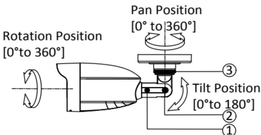
Figure 2-18 3-axis Adjustment
