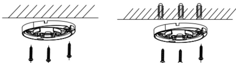
Figure 2-8 Attach the Mounting Base to the Ceiling
