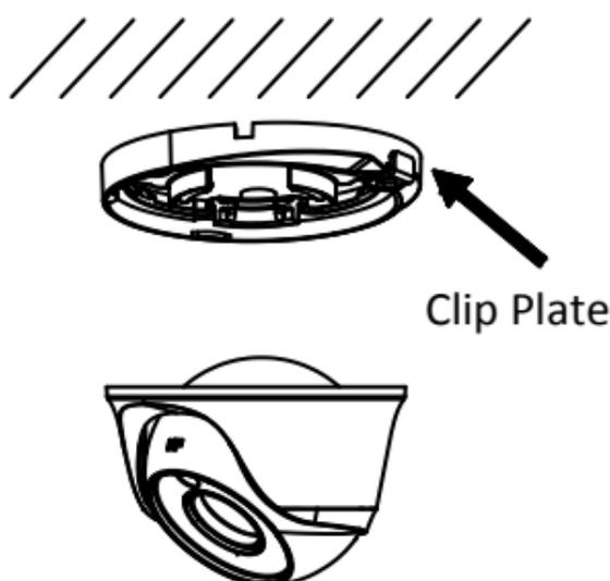
Figure 2-9 Secure the Camera with Mounting Base
