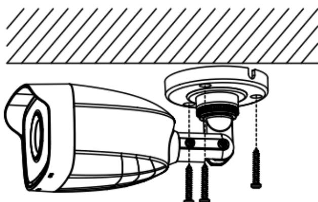
Figure 2-17 Fix the Camera to the Ceiling
