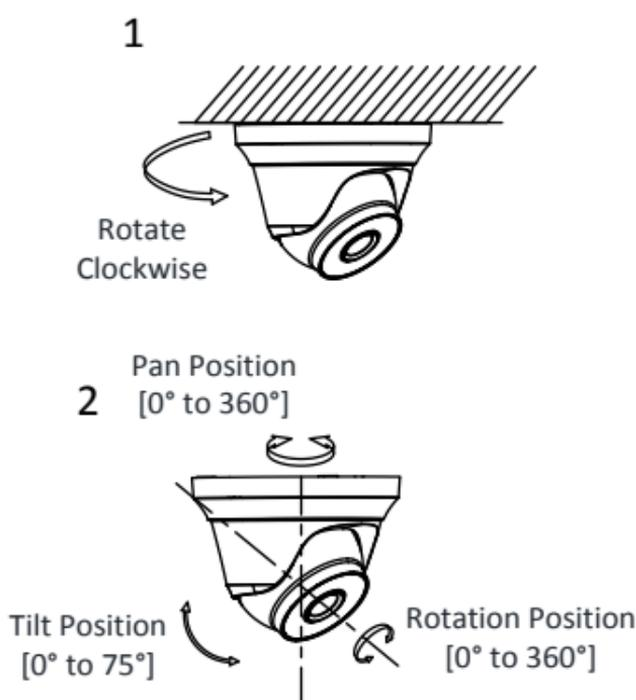
Figure 2-15 3-axis Adjustment
