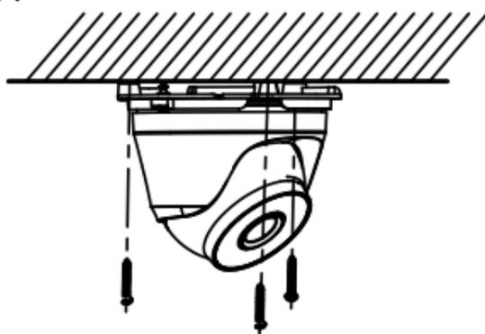
Figure 2-13 Attach the Camera to the Ceiling
