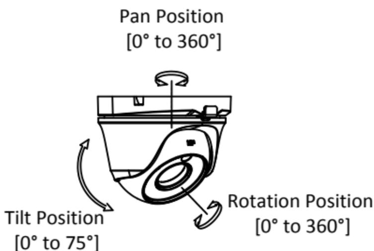
Figure 2-10 3-axis Adjustment
