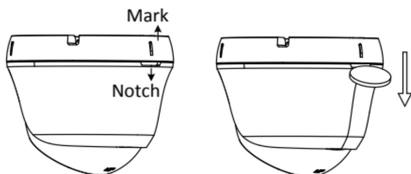
Figure 2-1 Disassemble the Camera
