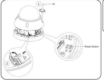
Note: For reset (used to return the camera settings to factory default mode), long press the Reset button for 8 seconds; the light turns off.
