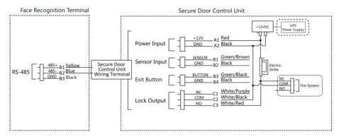
Figure 4-9 Wiring Diagram
