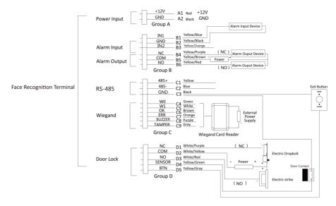
Figure 4-2 Device Wiring
