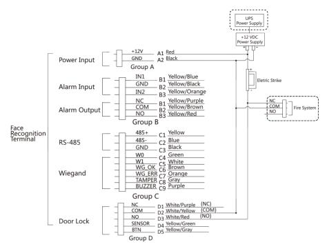
Figure 4-8 Device Wiring
