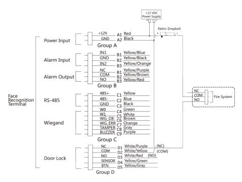
Figure 4-6 Wiring Device
