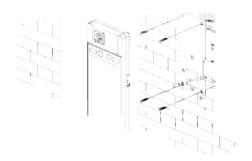
Figure 3-6 Install Device
