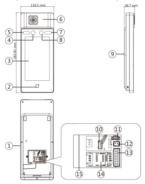
**Figure 2-1 Face Recognition Terminal Diagram**
