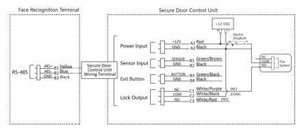
Figure 4-7 Wiring Secure Door Control Unit
