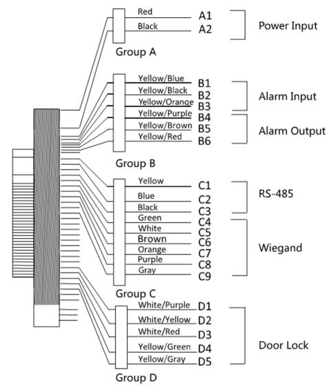
Figure 4-1 Terminal Diagram
