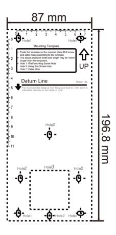
**Figure 3-3 Mounting Template**
