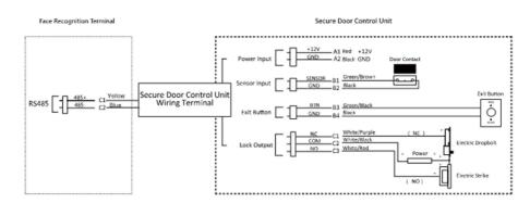
**Figure 4-3 Secure Door Control Unit Wiring**
