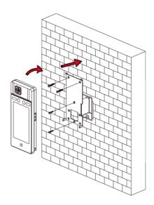
Figure 3-1 Install Device
