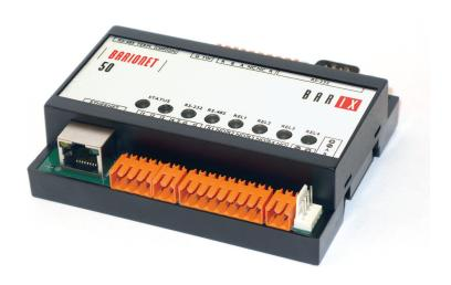
10/100 Mbit Ethernet connection, RS-232 and RS-485 serial interfaces, 4 dry contact inputs, 4 relays (30 V, 0.5 A), universal Dallas I-Wire® interface, Bus extension connector for additional I/O devices
