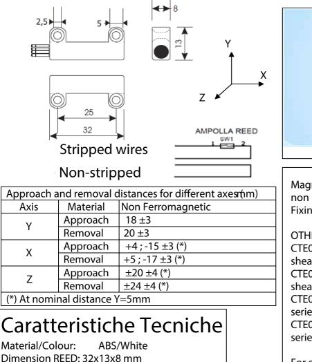
Dimension REED: 32x13x8 mm Dimension MAGNET: 32x13x8 mm Tmin/max: -25/+60°C Wiring: 4 white wire x 0,22mmq 30 cm long Approvals: EN50131-2-6 Grade 2 Class IV Certificate: IMQ CA12.01245 CEI 79/2 IMQ 1°Liv U0526
