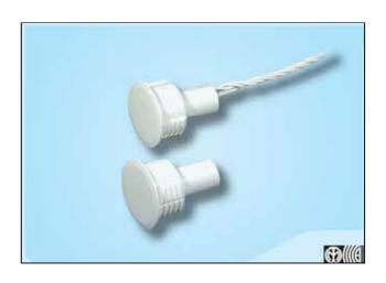
Flush fitting contact with ABS housing. Note: suitable for ferromagnetic surfaces. Drilling diameter 20mm, depth 29mm Where is possible Y=5mm mounting gap is recommended.
