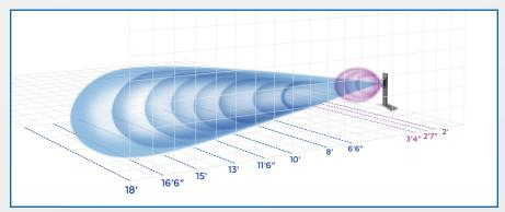
Microwave detection patterns (blue above) are adjustable from 7' to 18'. The Ultrasonic Sensor is for close range detection (purple). The OVS-01GT also features 5 sensitivity settings.
