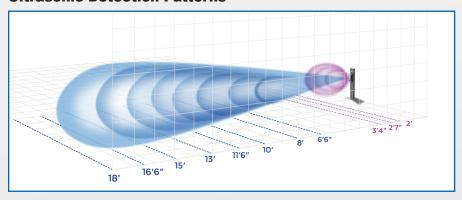
Microwave detection patterns (blue above) are adjustable from 6'6" to 18'. The Ultrasonic Sensor is for close range detection (purple). The OVS-01GT also features 5 sensitivity settings.
