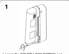
Loosen the COVER LOCK SCREW and remove the FRONT COVER. Do not touch the LENS surface.
