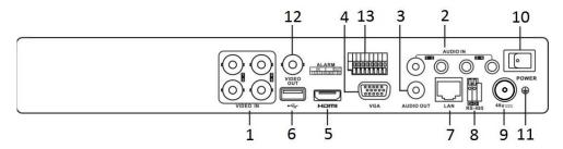
\*: The rear panel of DS-7208/7216HUHI-K2/P provides 8/16 video input interfaces.
