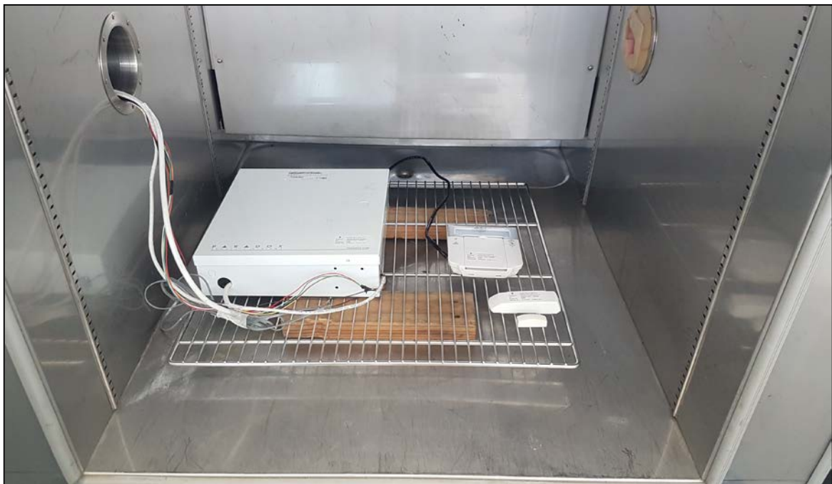
Photograph 6.1.1 The operational EUTs in the testing chamber
