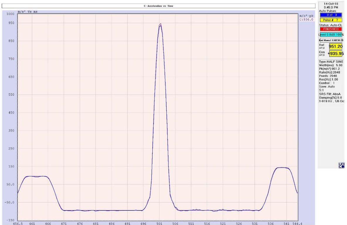
Plot 6.7.1 The positive shock pulse along transverse axis (operational) - Keypad
