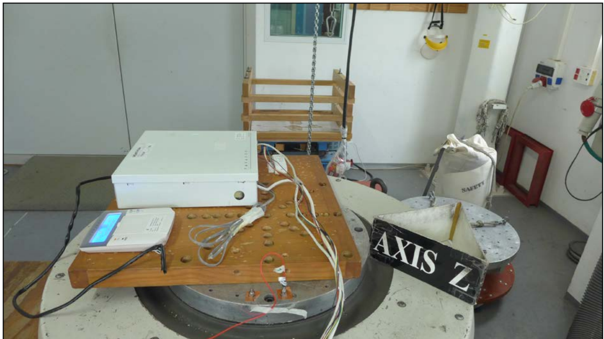
Photograph 6.6.1 Sinusoidal vibration test setup (vertical axis)
