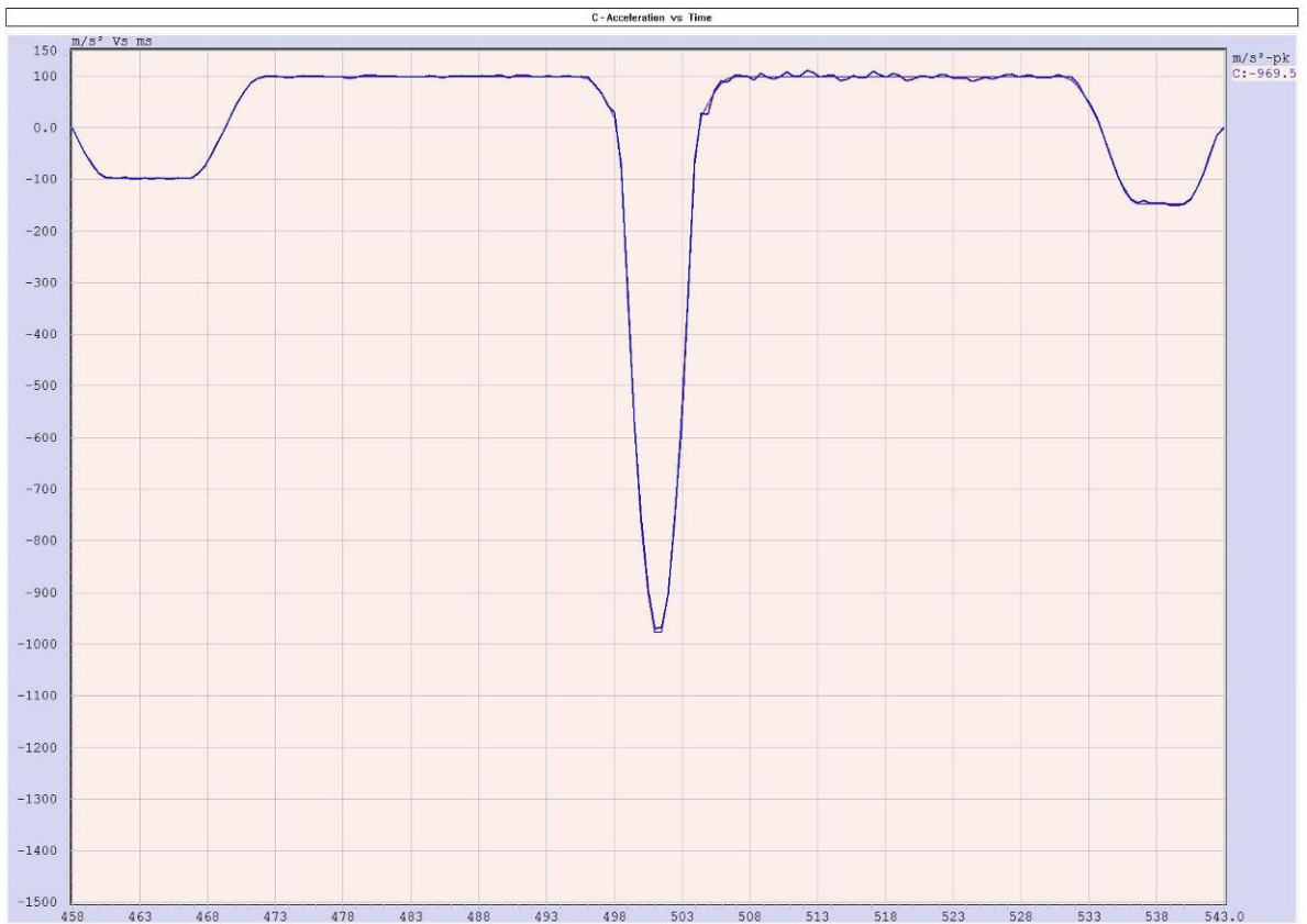
Plot 6.7.8 The negative shock pulse along longitudinal axis (operational)
