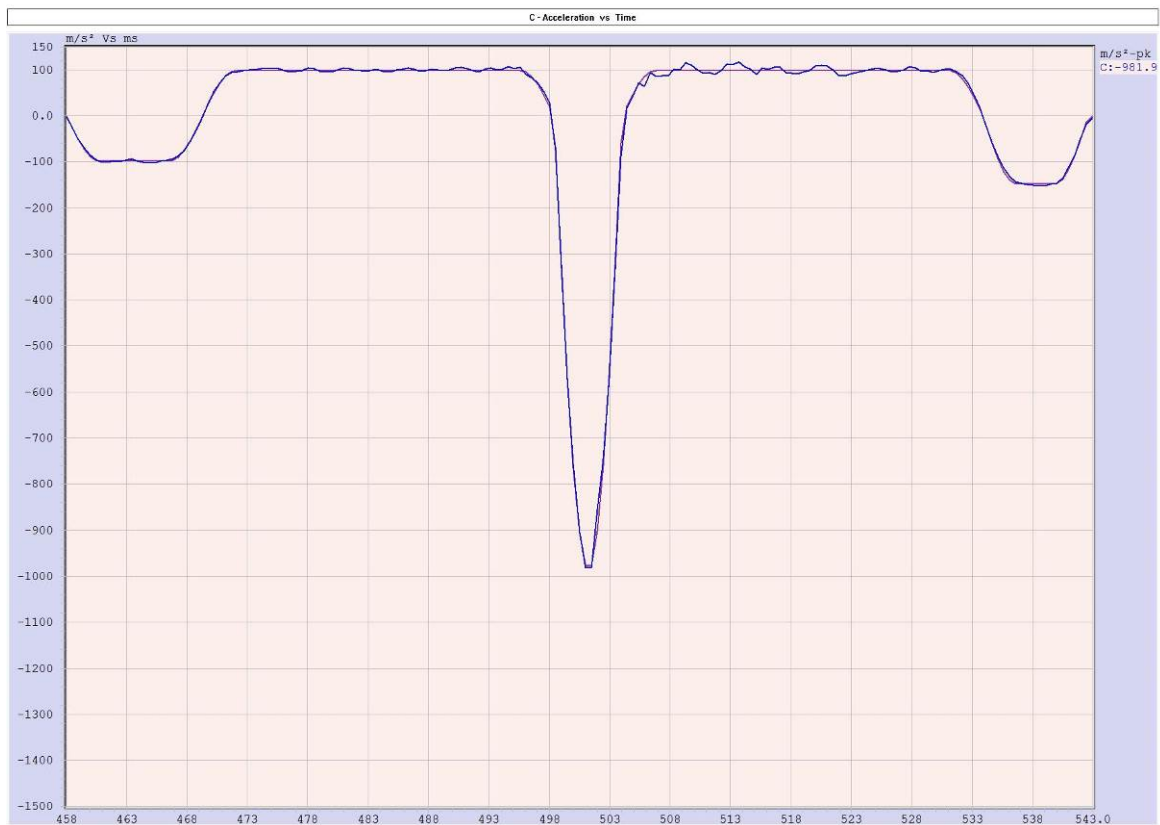
Plot 6.7.6 The negative shock pulse along transverse axis (operational)
