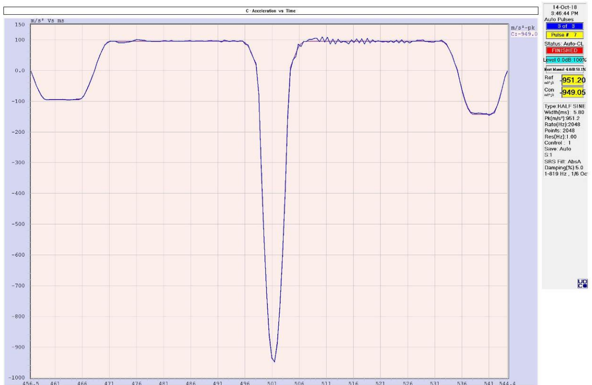
Plot 6.7.2 The negative shock pulse along transverse axis (operational) - Keypad
