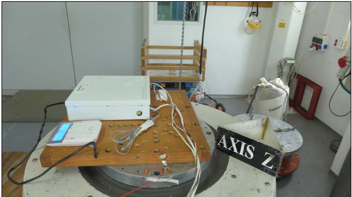
Photograph 6.5.1 Sinusoidal vibration test setup (vertical axis)
