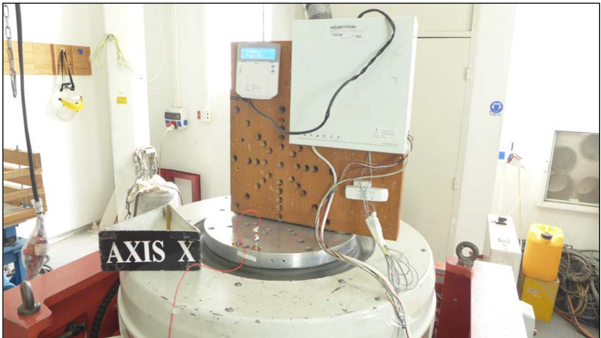
Photograph 6.5.2 Sinusoidal vibration test setup (transverse axis)
