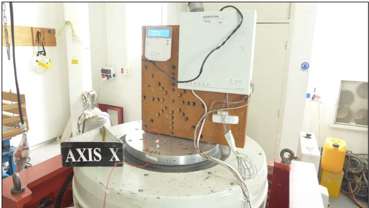
Photograph 6.6.2 Sinusoidal vibration test setup (transverse axis)
