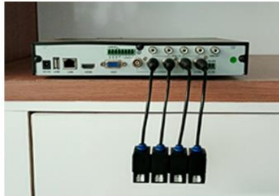
Baluns click together for a neat installation
