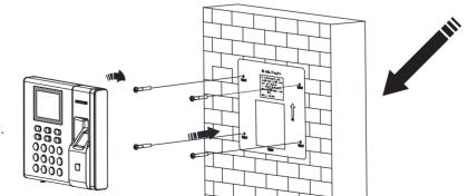
4. Align four holes of the device rear panel with the fixed screws and hang the device on the wall.
