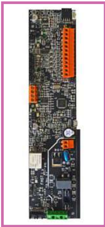
PLUS ELECTRONIC BOARD THAT EQUIPS PUMP PRO PLUS FOGGING SYSTEMS
