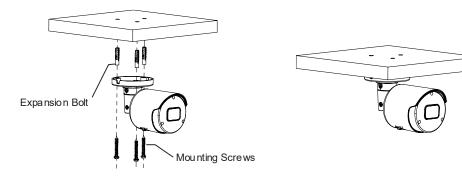
Insert 3 expansion boots into the ceiling and fix the equipment with 3 mounting screws.
