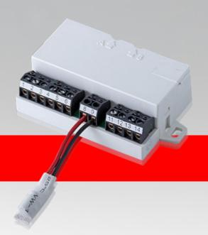
The single line conventional interface module is designed to integrate conventional fire detectors (maximum 32 pcs.) in the signal loop of the IFS002 panel. The built-in short-circuit isolator improves the signal loop reliability.
